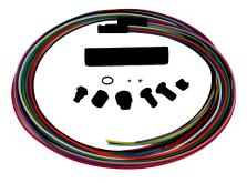
TLC Fan-out kits are designed for the quick and simple termination of loose tube (bare fiber) products. The three unique clips (included) accept different tube sizes including ribbon, 2mm and 3mm. 12 standard colors of the  $900\mu$ m Hytrel® tubes allow for easy identification of fibers.
