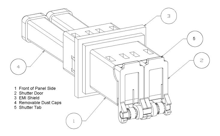
Installation of this adapter in a panel is accomplished by holding the Front side of the adapter (1) and pushing the opposite side through the hole, from the front side of the panel, until it latches.
