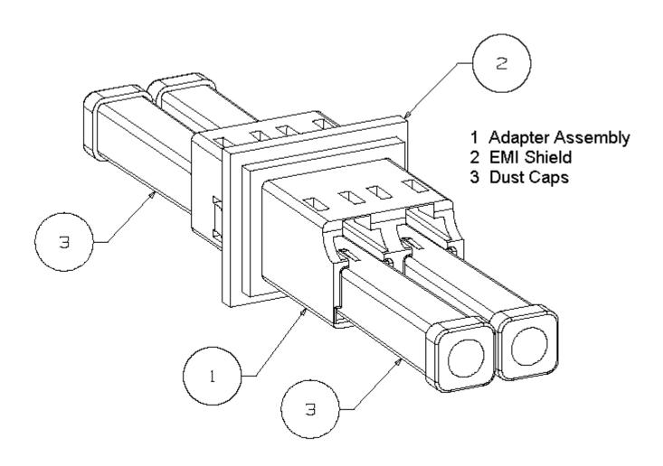
Installation of this adapter in a panel is accomplished by holding the Front side of the adapter (1) and pushing the opposite side through the hole, from the front side of the panel, until it latches.
