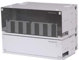
Combination shelf: One termination shelf and one splice shelf. The termination shelf can handle 96 (8 port panel) terminations or 72 (6 port panel) terminations. Shelves are available empty or equipped with (E/W) panels, adapters and splice trays.
