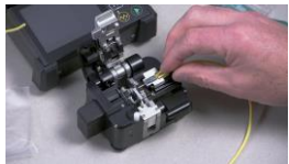
15. Clean the bare fiber with a cleaning wipe and fiber prep fluid. Clean the fiber.
