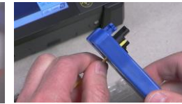
6. Ring cut and remove the outer jacket at 26mm.
