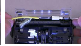
20. When the splicer beeps, the shrink process is complete. Confirm complete shrinkage of the protection sleeve.
