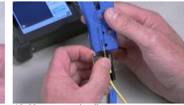
13. Use measuring line to ensure that exactly 7mm of coating protrudes from the extreme end of the holder.
