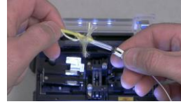
18. Slide the protection sleeve towards the ferrule housing unit. Make sure that the sleeve is covering the 900µm buffered fiber on both sides. Make sure the sleeve is against the housing.
