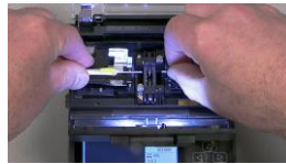
17. Remove the cord from the left cordage holder and release the ferrule from its ferrule holder on the right.
