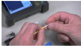
9. Slide the splice protection sleeve over the cord and aramid yarn.
