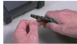
11. Remove the primary 900µm and secondary 250µm coating of the buffered fiber at 23mm.
