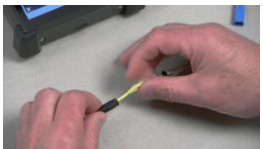
22. Put the aramid yarn tightly into the outer jacket then slide the stopper towards ferrule housing.
