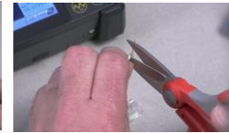
5. Remove the aramid yarn at 13mm.
