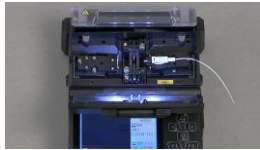
2. Load ferrule housing into the ferrule holder. Push until it clicks. Load the ferrule holder onto the right carriage of the splicer.
