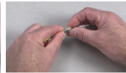
26. Spread the aramid yarn over the tail of the stopper and hold the aramid yarn in place by sliding the clamp over the outer jacket and aramid yarn.
