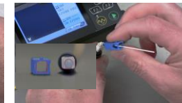
28. To complete the assembly, push the grip (with the direction of the same inner shape) onto the housing until it clicks.
