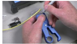
10. Mark the 900µm buffered fiber at 23mm. If the fiber is curved, mark on the back side of the fiber.
