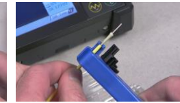
7. Split the outer jacket lengthways at 45mm.
