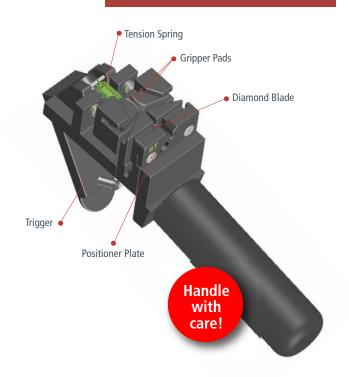
\* Diamond blade should be cleaned after every 20 cleaves, or more frequently as needed, to maintain cleave quality.  Holding the CLEAVING TOOL in a horizontal position, grip the handle while leaving your index finger free to actuate trigger.
