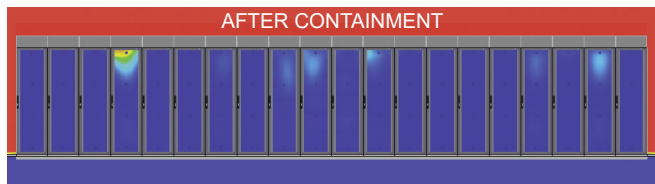
CFD analysis shows evenly distributed temperatures and reduced hot spots after the installation of Rack Top Angle Baffles in the cold aisle.
