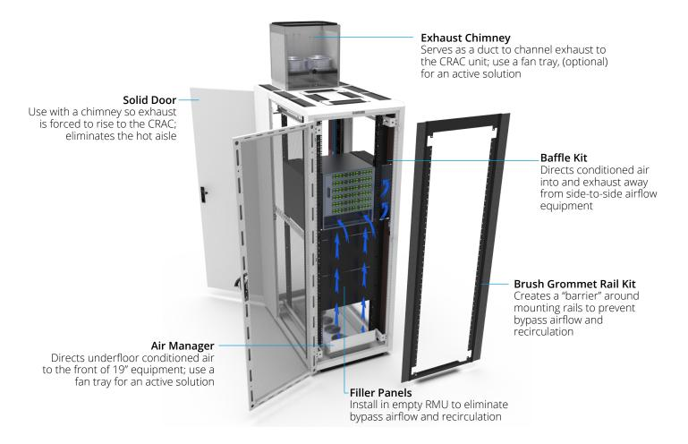
Flexible and scalable accessories for the ES address airflow at the cabinet level and throughout the data center. Implement best practices in the cabinet by using simple accessories to reduce bypass airflow and exhaust recirculation. Efficient airflow in the cabinet lends itself to an improved data center strategy that utilizes localized containment or hot aisle/cold aisle solutions—all designed with containment products that are built-to-order to ensure the best fit, function, and installation.
