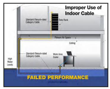
Standard indoor rated cables should not be used in conduits that are below grade or in the slab. These are considered wet locations. Indoor rated cables are not resistant to water penetration. Water in or adjacent to these cables will negatively impact electrical performance and prevent proper data transmissions.
