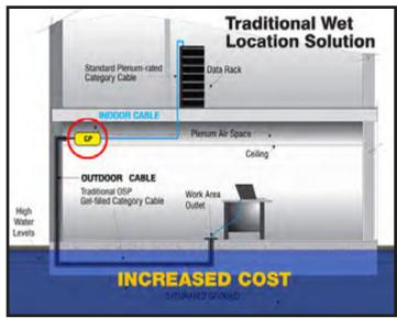
Outdoor (non-rated) cables are often used for below grade and in-the-slab applications. In these instances, the outdoor cable must transition to the appropriately rated indoor cable, such as plenum or riser, upon entering the building interior. This method of using two types of cable requires additional materials and labor as well as space for the consolidation point (CP).
