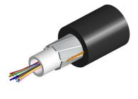
Outdoor Fiber Optic Cable, 24 fiber, OS2, LDPE, loose tube, gel-filled
