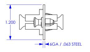
UNLESS OTHERWISE SPECIFIED DIMENSIONS ARE IN INCHES TOLERANCES ARE: TOLERANCES ARE: PRACTIONS DECIMALS ANGLES  $\pm 1/32$   $\times XX = \pm .03$   $\times 1^{\circ}$   $\times XX = \pm .010$  ALL FLATS TO BE  $\pm .005$
