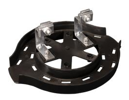
There's no reason to be concerned about weight and load conditions as the Sno-Shoe® is extremely lightweight. An empty unit weighs 8lbs. even with three loops of typical armored cable; with 288 fiber cable the total weight would still be less than 15lbs. If loading is still an issue, these storage units can be mounted vertically to consume less surface area.
