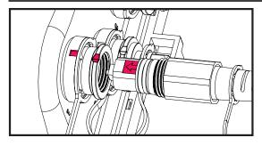
2.1 Align **arrow** on top of Surelight Connector with the **notch** on fiber access bulkhead.
