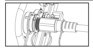
3.1 Insert H IP connector into fiber access bulkhead. If the H IP connector does not fully insert into the bulkhead, rotate connector slightly to either side until connector slides into place. DO NOT USE EXCESSIVE FORCE TO SEAT CONNECTOR OR DAMAGE TO THE PRODUCTS MAY OCCUR.
