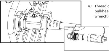
4.1 Thread connector coupler into the fiber access bulkhead and tighten (without use of a 216 tool or can wrench) until coupler is secured into the bulkhead.
