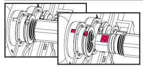
When removing the H IP connector out of the fiber access bulkhead, unscrew the connector coupler, pull the connector "straight out" of the fiber access bulkhead. If pulled out on an angle, damage to the bulkhead or connector may occur. Once removed, replace the dust cap into the fiber access bulkhead and seat to ensure proper sealing.
