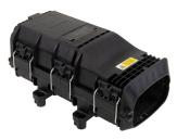
OFDC B8G Fiber Optic Splice/Patch Closure, Gel Cable sealing, 6 preinstalled 12 fiber trays , 8 duplex LC/APC adapters, 2x 1-8 splitter preconn at drop side
