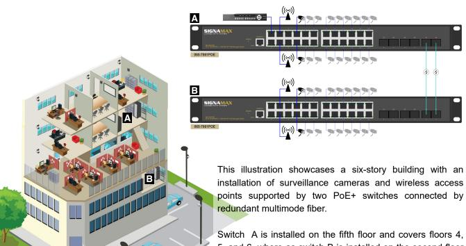
5, and 6, where as switch B is installed on the second floor provides coverage for floors 1, 2, and 3. The NVR connected to the PoE+ switch on the 5th floor receives all video feeds from cameras connected to both switches. Thus ensuring no SPOF.
