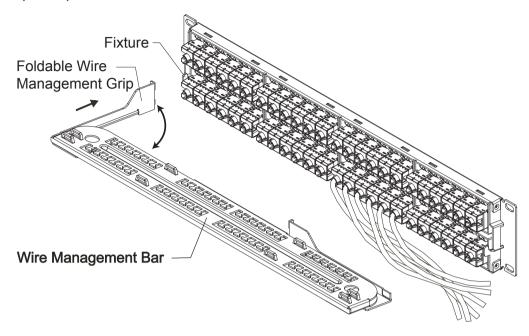
5. Fix the Solid Cables to the Cable Fixture Hole by Cable Ties
