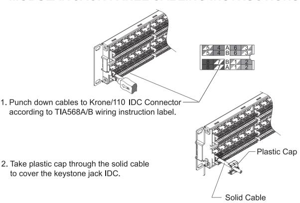
3. Insert the provided cable tie through the plastic cap and group this installed cable together.
